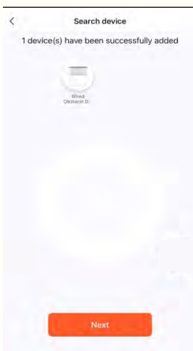
9) Briefly press Pair-key 4 times, and long press it 3s (shutter jogs once at 1s, and jogs again at 3s), or press transmitter S2 3 times and shutter jogs once, then click "Next".
