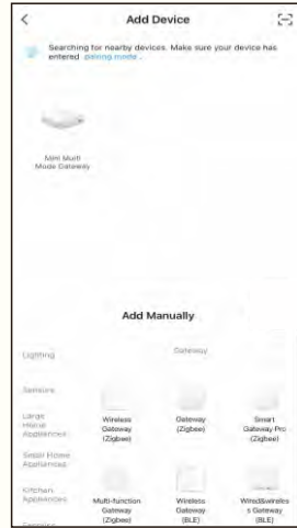
3) Add by automatic search or on this page click "Add Manually" — "Gateway control" — "Wireless Gateway(Zigbee)".
